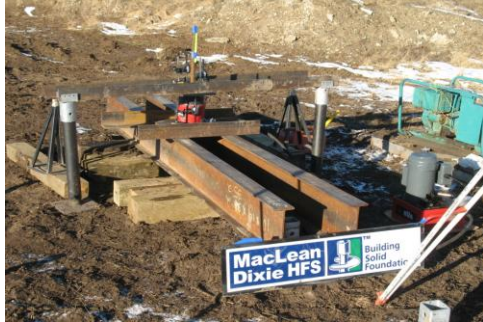
Full scale field testing-compression/tension/lateral
